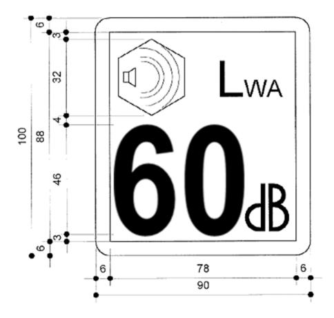
If the indication is reduced according to the size of the equipment the proportions given in the above drawing must be respected. However, the vertical dimension of the indication should, if possible, not be less than 20 mm.
